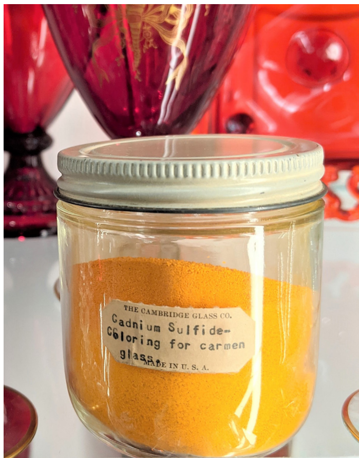
Cadmium Sulfide coloring for Carmen glass
