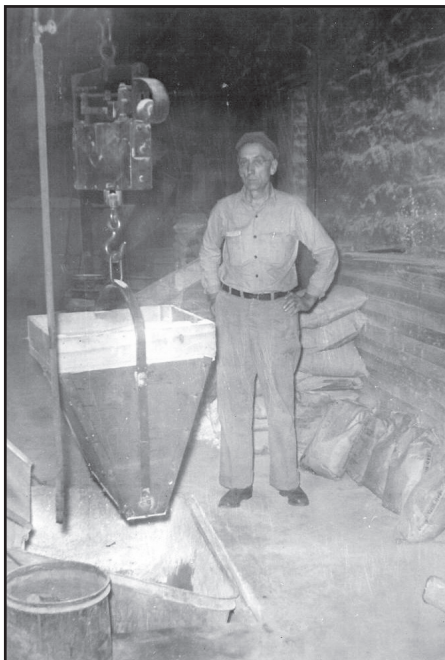
Cambridge Glass Company worker, George Sidenar, weighs material in a "hopper" which was attached to a large scale in the basement of the factory. This material would then be added to the batch.
